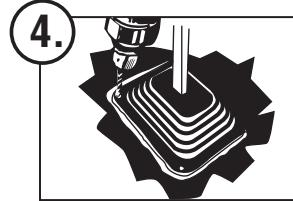
Slide the boot over the stick. Drill 1/8" diameter holes through floor using the boot holes as a guide.
