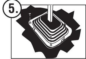
Position retainer plate into place and fasten with sheet metal screws supplied in package.
